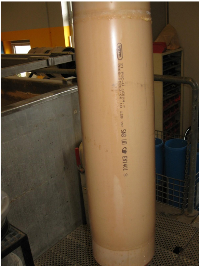
Sun whitened pipe after the pressure test of 1300 hours.
