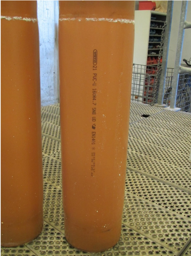
Fresh pipe after the pressure test of 1300 hours.
