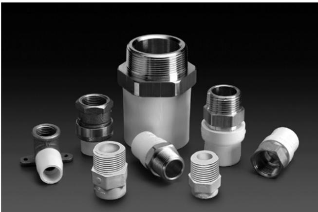
Transition fittings are available for connecting to other materials, valves and appurtenances and must be used for all hot water line connections. For cold water connections, male CPVC threaded adapters may be used. They are not recommended for hot water use as wide temperature fluctuations can result in a drip leak.
