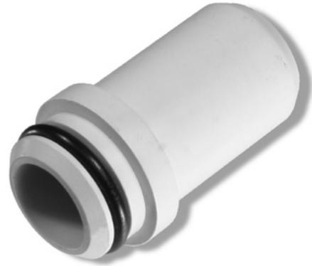
Standard compression fittings which utilize brass ferrules can be used on CPVC, although we recommend the use of an O-ring transition (above). If a brass ferrule is used, Teflon® tape must be applied over the ferrule to compensate for the dissimilar thermal expansion rates of the brass and CPVC that could possibly result in a drip leak. Care should be exercised not to over-torque the compression connection.
