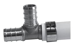
Ocenter the crimping tool exactly over the ring, and keeping both the ring and the tool square with the tube, close the tool completely.
