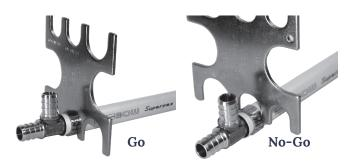
① Joints that do not pass the gauge check must be cut out and replaced. DO NOT RECRIMP (Double Crimp) THE SAME FITTING.
