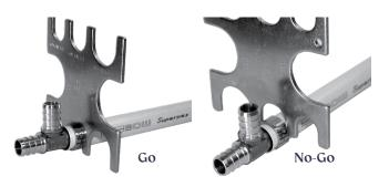
Joints that do not pass the gauge check must be cut out and replaced. DO NOT RECRIMP (Double Crimp) THE SAME FITTING.
