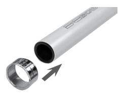
Insert a PEX fitting into tube up to the fitting shoulder and position the crimp ring 1/8" to 1/4" from end of pipe. To prevent ring from moving, squeeze the ring slightly with your fingers or a pair of pliers.
