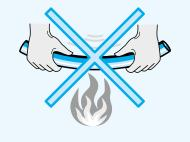
Pipeline cross-overs should be made with components designed explicitly for this purpose.
