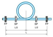
Compensation through modified pipeline routing
