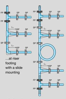
...by inserting a loop compensator
