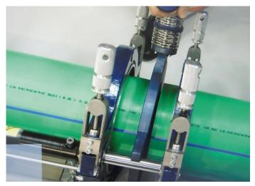
Heating with the heating plate
