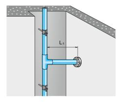
...allowing a certain degree of movement for the branch pipe in the wall pass-through point
