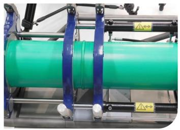
Cooling the weld seam
