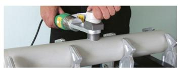
3/ Put the PP-RCT weld-in saddle on the adapter so that the mark on the saddle and the mark on the adapter are aligned. Heat-up the hole and the plastic weld-in saddle. The heating period is the same as with the 1" diameter (8 sec.). For weld-in saddle parts  $3-1/2" \times 1"$  and  $3-1/2" \times 1-1/4"$  the heating-up period is the same as for the 1-1/4" ones (12 sec.),  $4" \times 1-1/2"$  (24 s),  $4" \times 2"$  (24 s), see the table for socket fusion welding, page 30.
