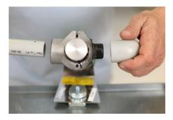
6/ The surfaces to be welded should be cleaned and degreased after the marking is complete. If this step is left out, then the melted layers may bond inadequately! Now you can begin the heating-up process.
