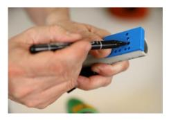
5/ Furthermore, it is recommended that you also mark the weld position on both the pipe and the fitting, in order to prevent the pipe from rotating after insertion. You can also use installation marks on fittings for the same purpose.
