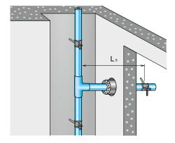
...creating a compensating length, allowing for vertical expansion at the riser
