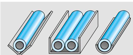
...by laying the pipe freely into a trough
