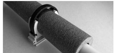
For hot water, the clip must be one size larger than the pipe (needs to be fitted over the insulation).
