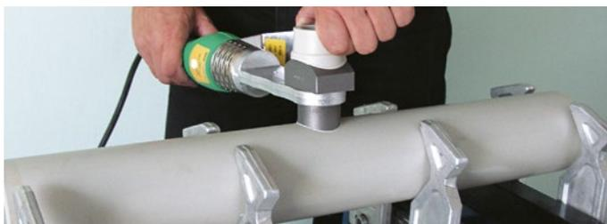
3/ Put the PP-RCT weld-in saddle on the adapter so that the mark on the saddle and the mark on the adapter are aligned. Heat-up the hole and the plastic weld-in saddle. The heating period is the same as with the 1" diameter (8 sec.). For weld-in saddle parts 3-1/2" x 1" and 3-1/2" x 1-1/4" the heating-up period is the same as for the 1-1/4" ones (12 sec.), 4" x 1-1/2" (24 s), 4" x 2" (24 s), see the table for socket fusion welding, page 30.
