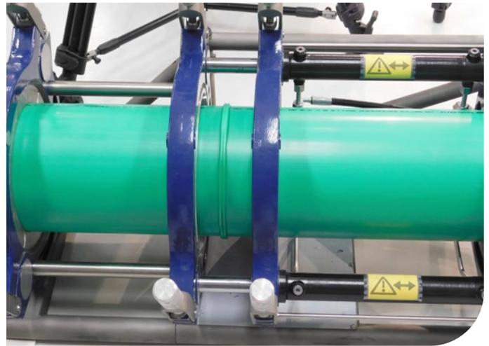
Cooling the weld seam
