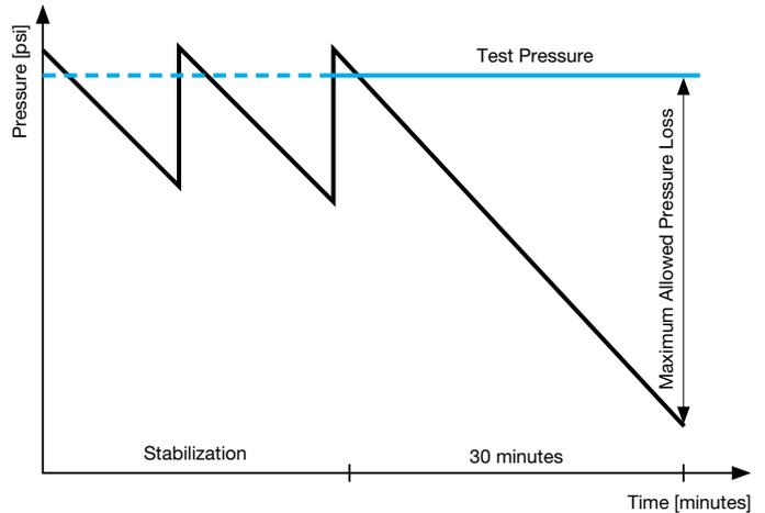
Max. Allowed Pressure Loss = 9 psi for SDR 7.4, SDR 9 a SDR 11
