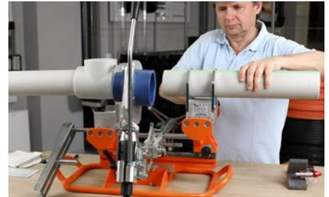
Fixing and aligning the components, then heating them up
