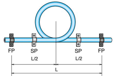
Compensation through modified pipeline routing
