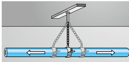
...by pipe-straps suspended on hooks
