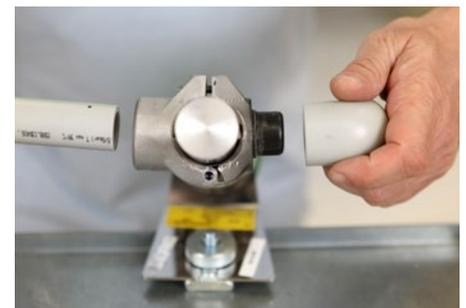
6/ The surfaces to be welded should be cleaned and degreased after the marking is complete. If this step is left out, then the melted layers may bond inadequately! Now you can begin the heating-up process.
