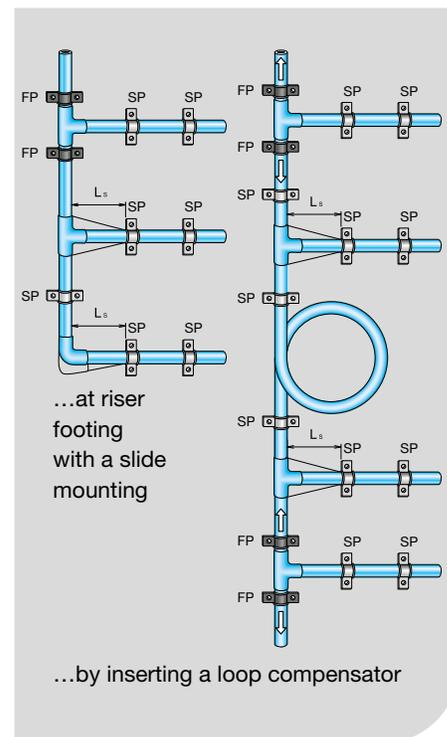
If it is necessary to divide the riser into several expansion sections, then it can be achieved by placing fixed points. The riser fixed points are always fixed under and over the T-pieces at a branch pipe or a socket, which also prevents the riser from falling. The pipe expansion must be accounted for between these fixed points.
