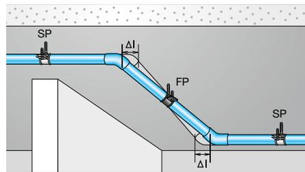
Compensation through modified height of the pipeline
