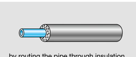
...by routing the pipe through insulation under plaster (flush-mounting)
