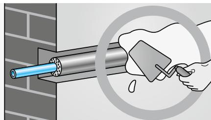
If water supply / distribution piping systems are installed inside stack partitions, they must be fixed in a suitable way – such as with a system of metal clips and supporting elements.
