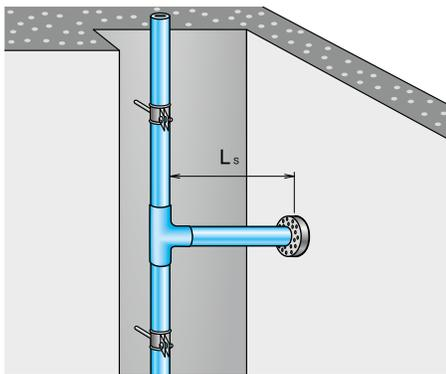
...allowing a certain degree of movement for the branch pipe in the wall pass-through point
