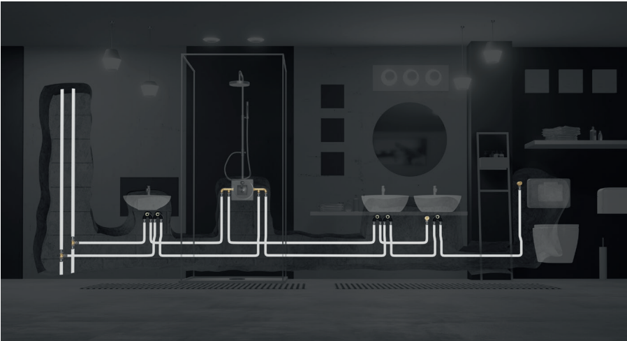
Fig. 43: In series installation.
