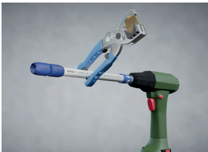
Fig. 23: Calibrating the pipe.
