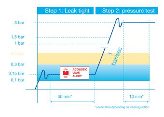
Fig. 28: Pressure test protocol when testing with air.
