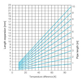
Thermal Linear expansion of.Wavin multi-layer composite pipes (based on  $\alpha$  = 0,025 mm/m.K)
