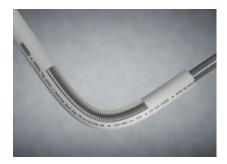
By bending the pipe the demand of fittings needed for the installation can be reduced. The pipe is easy to bend: by hand, with the aid of the bending spring or using the Wavin bending pliers. Bending springs and bending pliers are preferred to be used to ensure the pipe is not kinked by accident. Larger diameters can be bend with pliers with appropriate dimensions, bending radius min. 3xDa.
