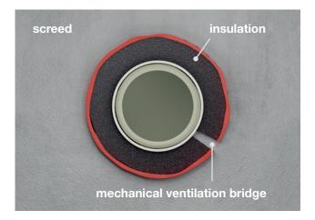
Fig 35: Mechanical vibration transmission through defective pipe insulation.
