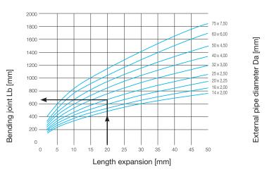
Fig. 32: Bending joint classification of Wavin multi-layer composite pipes.
